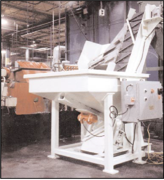
• Parts in dump hopper were interlocking. An SCR-100 on hopper separated them
