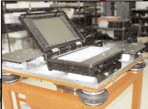
• SCR-350 on Test Table testing computer parts
